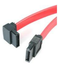
The SATA18LA1 Left Angle (90-degree) SATA Cable features a standard (straight) SATA receptacle as well as a left-angled SATA receptacle, providing a simple 18-inch connection to a Serial ATA drive, with full SATA 3.0 bandwidth support of up to 6Gbps when used with SATA 3.0 compliant drives.
