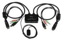
The SV211HDUA 2-Port HDMI® Cable KVM Switch with Audio and Remote Switching Control lets you control two HDMI, USB equipped PCs with a single monitor, keyboard, mouse and audio peripheral set.
