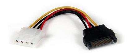
The LP4SATAFM6IN SATA to LP4 Power Cable Adapter features an LP4 female power connector and a male SATA power connector, allowing you to connect an IDE hard drive to a Serial ATA power connector provided by the computer power supply.
