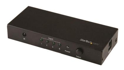
This 4-port HDMI video switch lets you share an HDMI 2.0 display or projector with four HDMI 2.0 video sources. The switch features four independent video inputs that can each support 4K resolution at 60Hz, making it the perfect solution for connecting four video sources to a display that has a limited number of HDMI 2.0 ports.
