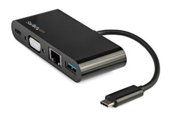
Expand the connectivity of your USB-C<sup>™</sup> laptop with this USB-C VGA multiport adapter. It connects to your USB-C or Thunderbolt<sup>™</sup> 3 port to add VGA video output, a USB 3.0 (Type-A) port with Fast-Charge capability plus a Gigabit Ethernet network connection. Mac, Windows® and Chrome OS<sup>™</sup> compatible, it's the ideal accessory for your MacBook, laptop, tablet, Chromebook, smartphone or other USB-C device (with support for DisplayPort Alt Mode).
